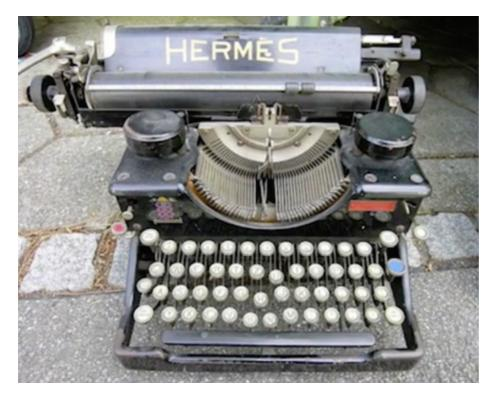
When the key is pressed, it swings a lever with the corresponding character and inks it onto the page, which looks like this.
