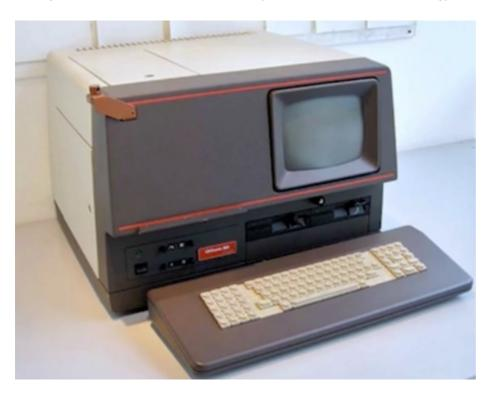
The image above is the CRTronic 360. This is called a photo-type setting, which means it projects light through a film negative of an image of an individual character, and all the photographic paper collects in a spool.
