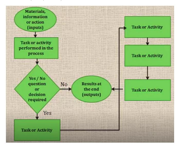
Notice, we have the oval to start, which includes the inputs. Some kind of action is required because the process is starting with this oval.
