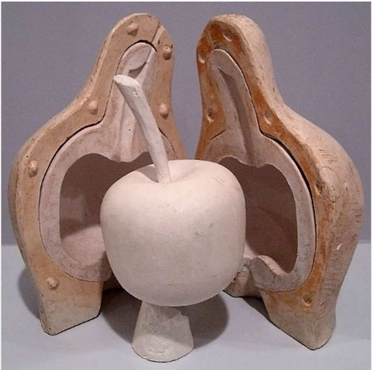
Lost Wax Casting of an Apple in Plaster
