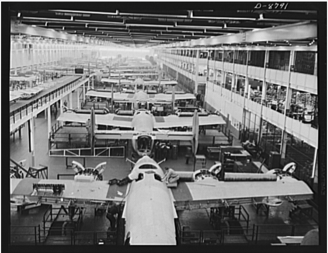
An assembly line for B-24E Liberator bombers at Ford's plant in Willow Run, Michigan, 1943. Assembly line technology helped the U.S. quickly begin building the weapons it needed to fight World War II.
