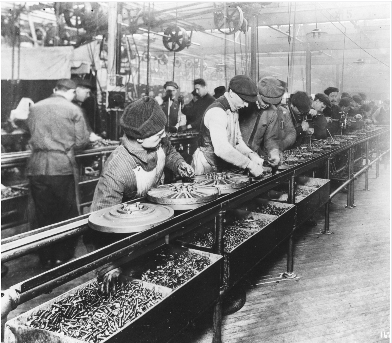
Workers on the first moving assembly line put together magnetos and flywheels for 1913 Ford automobiles in Highland Park, Michigan
